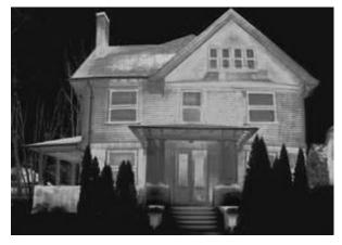
An energy audit done with the aid of thermography (infrared scanning) can help detect thermal defects and air leakage in your home.
