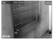
The picture on the right shows infrared imaging on a window.
